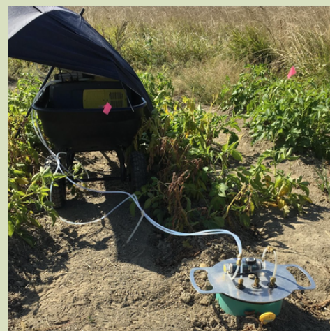
Figure 4. Using a gas analyzer to measure greenhouse gas emissions. Photo by the research team.
