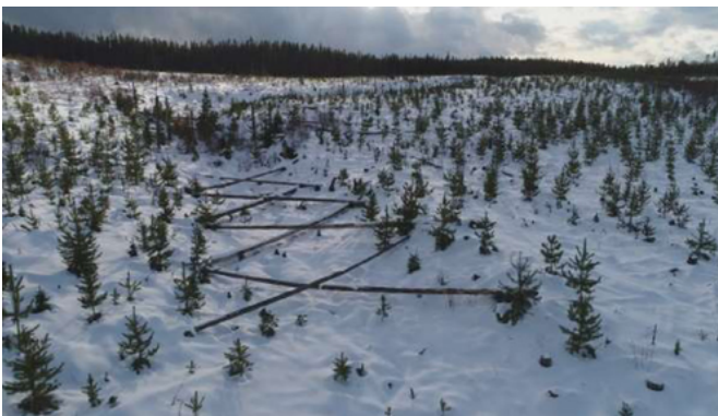
Figure 2. For the set-up, eight logs were laid on top of the stream in a criss-cross pattern. Photos by Clayton Bradley.
