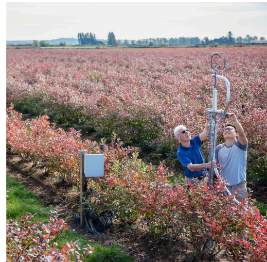
Figure 1. Researchers Patrick Pow and Andy Black adjusting the sonic anemometer, used to measure wind. Photo by Martin Dee.
